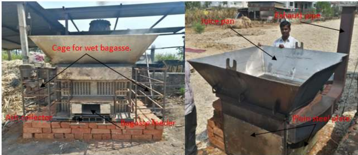
Fig.1 Modified portable jaggery plant
